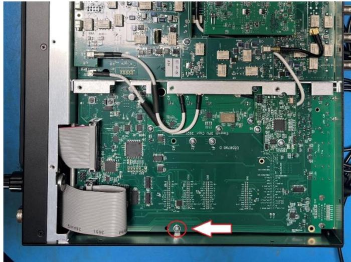
*Photo 3. If your K4 has a brazed bracket, remove this screw before lifting off the side panel.*
