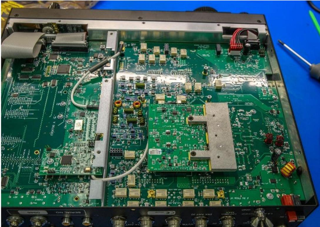
*Photo 11. K4 underside before Subreceiver is installed.*
