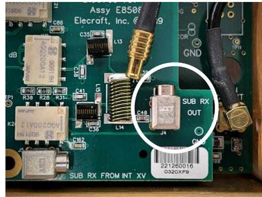
*Photo 13. Coax Jumpers. Subreceiver antenna (left), DDC (right)*
