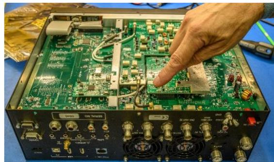
*Photo 12. K4D with Subreceiver board and coaxial jumpers installed.*
