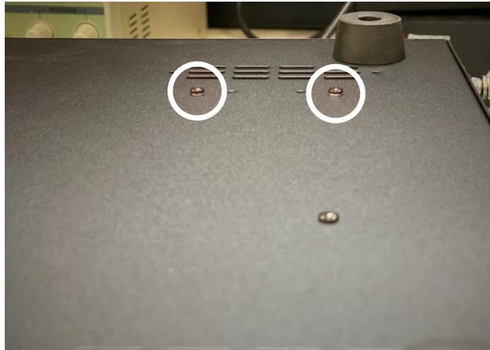
*Photo 1. Two lock washers secure the LPA heat spreader to the bottom cover. These are critical for heat dissipation.*
